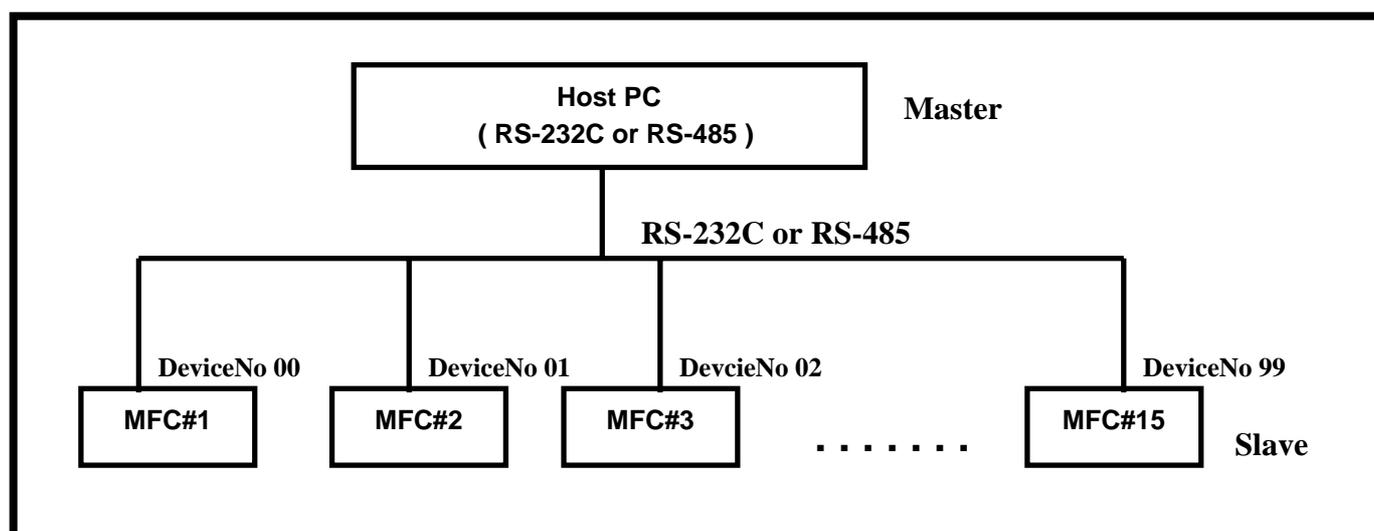
Fig.1 diagram of connections (Host PC – MFCs)
